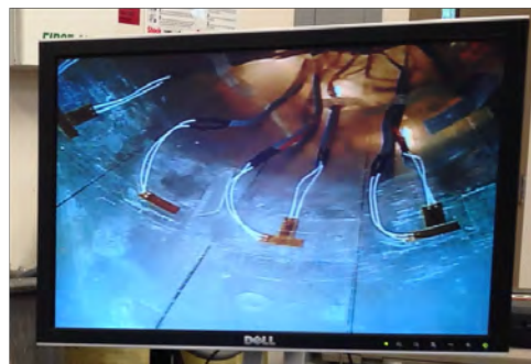
Figure 2.9: Installation of strain gauges inside and outside of the pipe.
