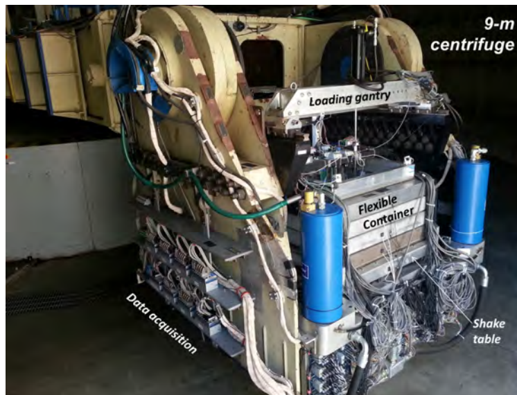
Figure 2.3: Configuration of the instrumented container mounted on the 9m-radius centrifuge arm (CGM, personal communication).
