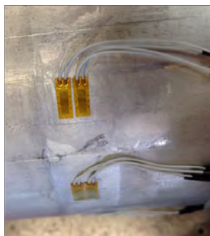
Figure 2.9: Installation of strain gauges inside and outside of the pipe.
